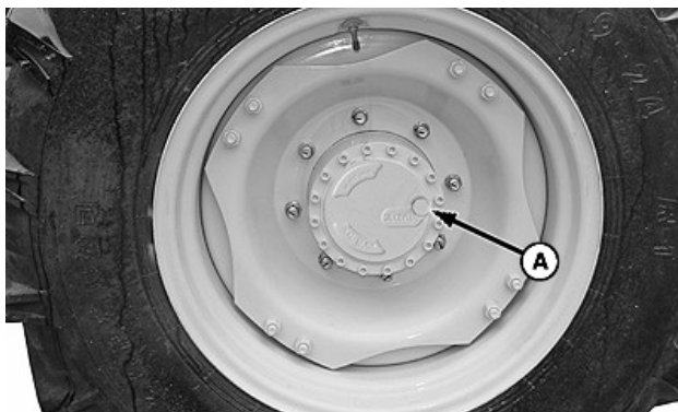
Position to Fill (for 6095B and 6110B tractors)
